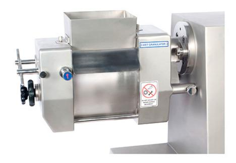
This machine is equipped with an oscillating rotor suitable to manufacturer wet granulates of various granule sizes. Sieves are easily exchangeable. Rotor, sieve and all parts coming in to contact with the material are constructed of stainless steel. Each apparatus is supplied with one sieve. The following mesh sizes are available for the wet granulator on request. 6 mesh to 50 mesh.
