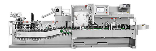
HC 200 is a horizontal carton packaging machine in a continuous / intermittent motion. This model is suitable for small and medium sized production, in which is capable of producing 200 cartons per minute. By designing the main working station as the combination of both servo and mechanical systems, such design has guaranteed the operation speed with minimal maintenance.
