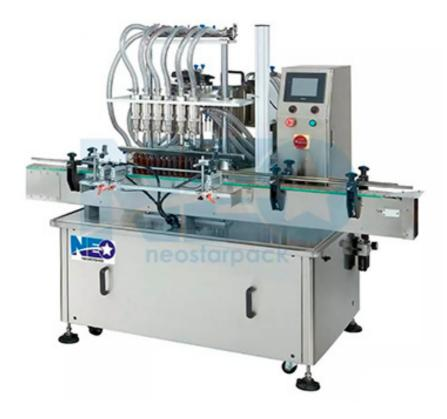
Automatic 6-nozzle overflow liquid filler FL4350 is best suitable for filling with foamy, flammable, corrosive liquid products, or products which require consistent filling level. The number of nozzles can be customized according to your needs, and the filler can also be connected with other packaging machines to build up a complete production line.
