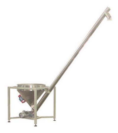
It is a free standing mobile screw elevator with an integral loading hopper. A rotating paddle inside the loading hopper loosens the hopper contents and assists the feed into the tubular screw elevator section. The screw then elevates the material and discharges it into processing or packaging machinery as required.
