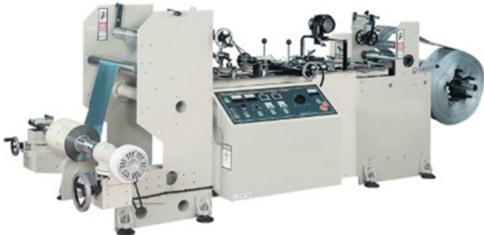
The AFK-250PVC is a versatile and economical plastic bag and shrink label production machine, ideal for center-seal plastic bags or shrink label sealing. Its simple design ensures easy operation and low maintenance, making it perfect for entry-level production lines. Equipped with an oscillating air expansion shaft for smooth rewinding, the machine requires only one operator, with optional cantilever or five-claw shaftless rewinders for flexibility.
