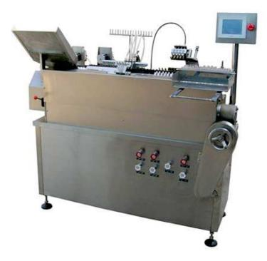
The machine is a new generation of the ampoule drawing, filling and sealing combined equipment for injections. It adopts the rectangular feeding instead of the traditional ampoule feeding methods. In such case, the feeding is steady with no easy broken ampoule. A modern clutch is mouthed under the ampoule feed hopper.
