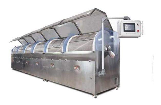
ZL300 intelligent soft gel tumbler dryer combines the working principle of common tumbler dryers in the market and the rotary dehumidifier this product was designed developed and tested 3 years ago. It is a totally new optimized and designed dryer this machine is the combination of shaping, drying and polishing.
