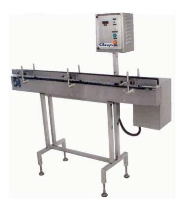
The slat conveyor belt is having stainless steel structure with moving S.S. slat chain of width 3  $\frac{1}{2}$ " in the center. Structure made out of S. S. square pipe & supported on adjustable bolts. Is useful to transfer container from one place to another place, without human touch which also reducing manual labors.
