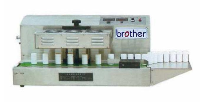
FL series portable induction sealing machine&Continuous induction sealing machine utilizes electromagnetic induction principle to produce instant high heat to melt aluminum foil that then adheres to the bunghole, teaching the aim of wet-proof, leakage-proof, mildew-proof and extending preservation time. Now it is widely used as sealing package machine in industries such pharmaceuticals, pesticides, lubricant and cosmetics etc.
