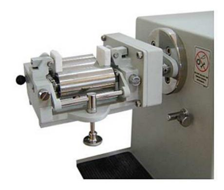
Triple Roller Mill – STRM is used in the preparation of ointments, salves, dough and similar products. The hourly production is from 2 Kgs. to 12 kgs. depending upon the constituency of the material. Three hard stainless still roller, which are 110 mm long, and 50 mm diameter produce the Rolling action.
