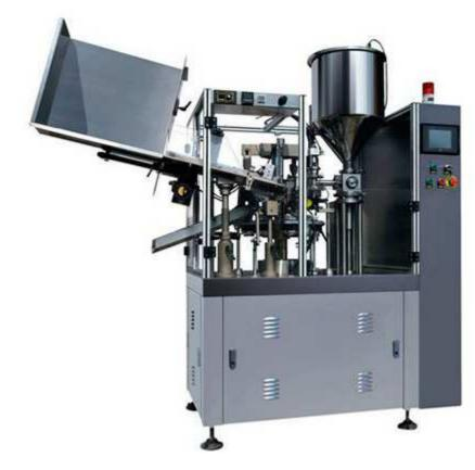
With easy and quick adjustment, it is suitable for using multiple kinds of soft tubes for filling. The part contacting materials is made of 316L stainless steel, clean, sanitary and conforming to CMP for medicine manufacture.
