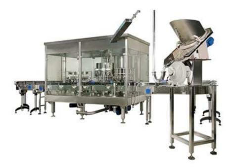
SMA Series Monobloc is designed for filling energy drinks and medical standard fluid in small glass containers. Its compact and stainless inclined machine table top design enabled high standard of food and micro biological safety to be achieved.
