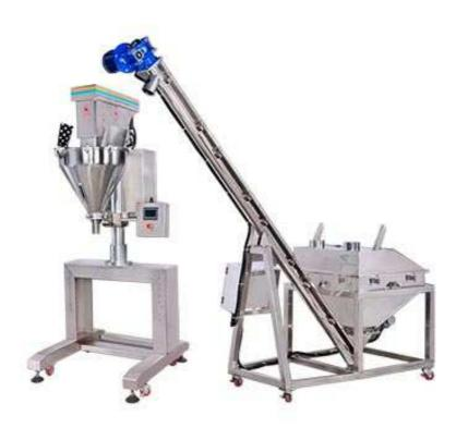
The GJ-2001 auger type metering filling machine is suitable for all types of free-flow and non free-flow powder and granular products.
