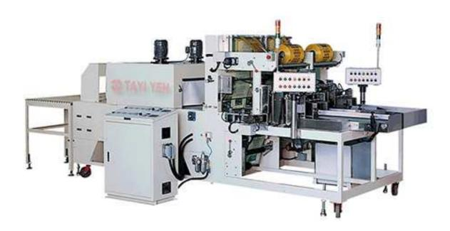
SA-106-2 is suitable for group packing bottles, such as water, beverage of canned food. Available with transparent PE shrink film (each Top and Bottom film cradle) OR printed PE film (only Top film cradle) Easily change the package matrix among modules. It contains two packing lanes, and its speed could up to 44 packs per minute based on 330ml can by package matrix of 3x2.
