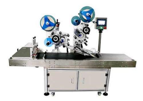
Dedicated to the thinner, lighter card products, we have achieved the integration of dividing cards, automatic labeling, and automatic card collection with the application of suction technology and suction belt conveyor that preventing deviation in the process of conveying, and improving labeling accuracy. such as: scratching cards, PE Bags, boxes, advertising color pages and other labeling.
