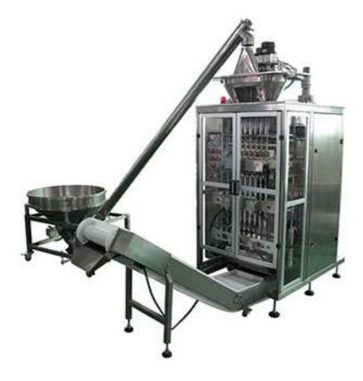
This automatic packaging machine can automatically complete the automatic measurement, automatic filling, automatic bag making (printable), sealing, fixed package cutting, etc.
