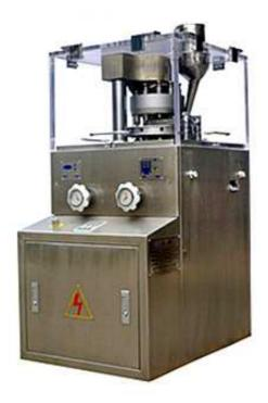
The machine is a single press type, continuous automatic tablet press for pressing granular raw materials into tablets. It is used for small scale production.
