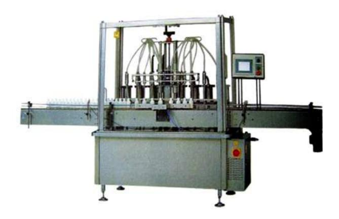
This machine is automatic quantitative thick paste filling machine can be used in the liquid, dilute viscous filling operations, applicable to all types of round bottles, flat bottles and other special-shaped bottles, the machine is designed with a linear movement pattern, Using PLC logic controller and various detection sensors and retractable cylinder to achieve automatic control purposes, there are bottle filling, no bottle no filling, no foam filling
