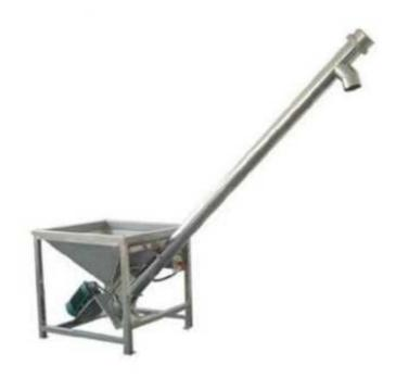
This machine is a automatic screw feeding machine, material is sent to the hopper by the rotary movement of screw (auger). Connected with level switch, it can feed automatically under the control of PLC. This machine can be used with our company's DXD series of powder filling packaging machine. It is the ideal auxiliary equipment.
