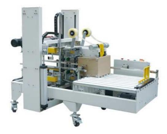
Automatic corner sealing machine can be used with other "one" type adhesive tape supporting the use of models. This box is suitable for carton size changes fast, specifications and more varieties of carton packaging use. When the carton size changes, the sealing machine automatically adjust the sealing width and height.
