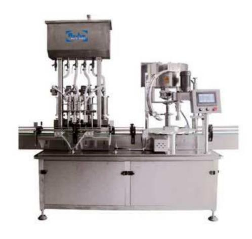
The equipment is automatic filling and capping machine, which makes the high-viscosity filling and ordinary pressure filling into one. Under the high-viscosity mode, the machine adopts the cylinder to control filling head so that it can ensure the stability and precision; under the ordinary pressure filling mode, the filling part adopts fixed passageway parameters, and the machine realizes the different filling dose by controlling the filling time.
