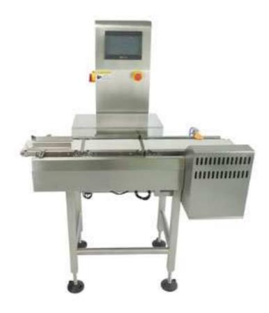
A checkweigher is an automatic machine for checking the weight of packaged products. The checkweigher is normally used to ensure that the weight of a pack of the product is within specified limits. Any packs that are outside the tolerance are taken out of line automatically. Checkweighers are widly used in clean rooms, mints (rolls of coins), dry atmosphere environments, wet environments, produce barns, food processing, drug processing, cosmetics filling, etc.
