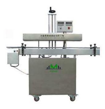
This automatic inductor plastic bottle Aluminum Foil Sealing Machine widely used in medicine, pesticides, lubricants and cosmetics industry.
