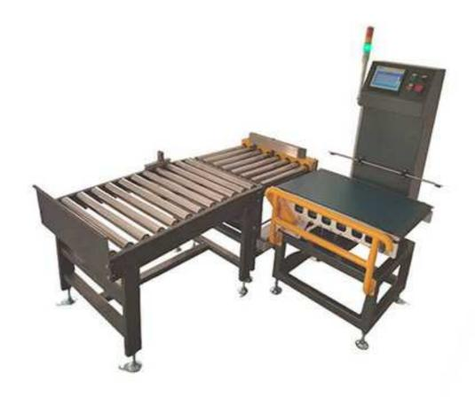
Check weigher with reject or mainly use for check carton weight or bag weight within a certain range you set and required. Check weight automatically and display on the LCD screen. And reject the carton or bag automatic which one is not in this range you set before.
