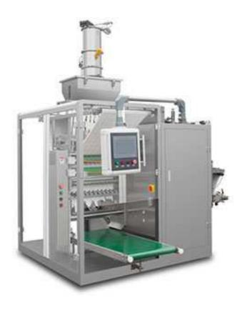
DXDK1200 Sachet Packing Machine with its compact structure is the leading machinery in China, which is used to pack pharmaceutical granule, powder and liquid, which is also can be used for food and cosmetic products. The machine meets GMP and CE Standard.
