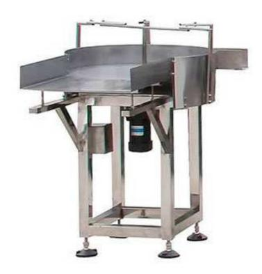
Automatic bottle feeding machine (also named rotary unscrambler) used in plastic jars and glass bottles. Its procedure: put bottles onto round turntable, then turntable rotate to poke and loading bottles to convey belt.
