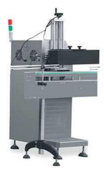
PLC control, operational memory and data saving, adjustable sealing duration and power, and overload protection.
