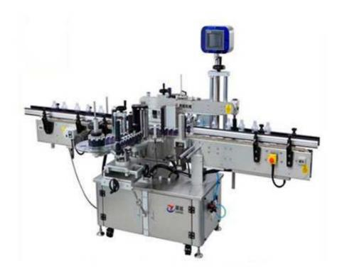
The front and back label applicator will labeling front and back side, or two adhesive label, one self-adhesive label on shoulder, one sticker label on body.
