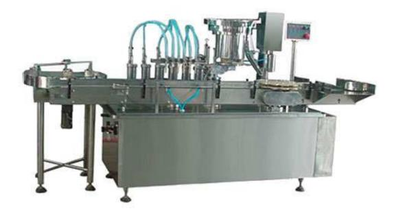
This monoblock filling and sealing machine is mainly used for filling, capping, and sealing 30-500ml bottles, and it is the major machine of oral liquid production line.
