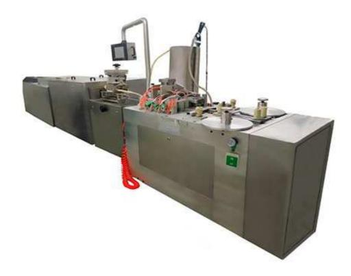
ZSBS-I model suppository filling and sealing machine that has been developed for the production of suppositories in PVC, PVC+PE. Its working is completely automatic, pneumatically based, controlled by a programmable logic (PLC).
