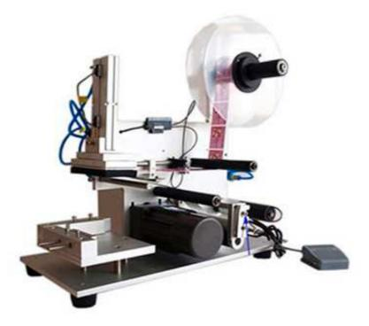
Suitable for different size of adhesive label or adhesive film on all kinds of flat bottle, High accuracy and high speed, dispensing & labeling automatically.
