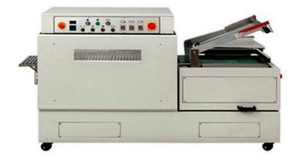
DFSC450 continuous seal-cut-shrink packaging machine combines work of seal-cut and shrink packing of film in one operation. Electric magnet absorbs cutting frame automatically when frame is pressed down. Then object is automatically transmitted into shrink tunnel through conveyor when film is cut. Therefore, it has high efficiency. It is suitable for packing boxes, toys, electronics and so on.
