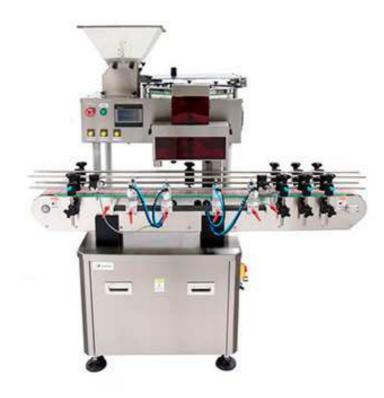
Automatic Tablet / Capsule Counting Machine TC-415 is designed for accurate counting and bottle filling of all kinds of tablets and capsules.
