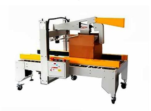
The machine is used to seal top and bottom tape of carton automatically. It has functions of coverfolding, tape sealing and feeding automatically. Economical and high efficiency. It is an ideal automatic carton sealing equipment.
