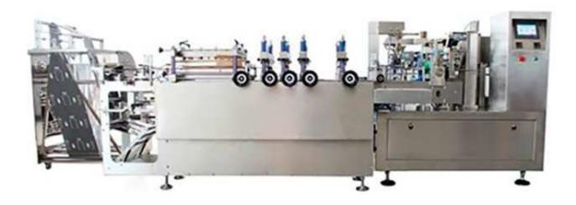
Form fills seal packaging main machine standard configuration and the advantage. The main devices on the machine and the advantages of the devices: All of the devices on the machine are independent and also could be quickly moved by a handle, so you don't need to change any devices on the machine if you change the size of the pouch, so the total time just need around 10 minutes.
