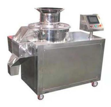
This rotary granulator is a device that uses a set of relatively rotating milling knives to squeeze the material out of the granules through a stainless steel screen. This machine can be combined with conveyors and drying equipment to form an automatic production line, saving labor costs.
