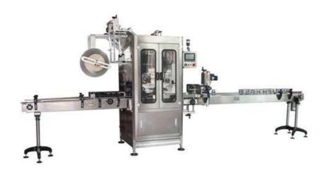
Shrink sleeve labeler applicators are mandrel style machines that use servo motion control to deliver consistent, repeatable performance. Container changeovers are tool-less and require less than ten minutes depending on product sizes and shapes. We also offers a full range of shrink sleeve applicators for low, medium and high speed production environments.
