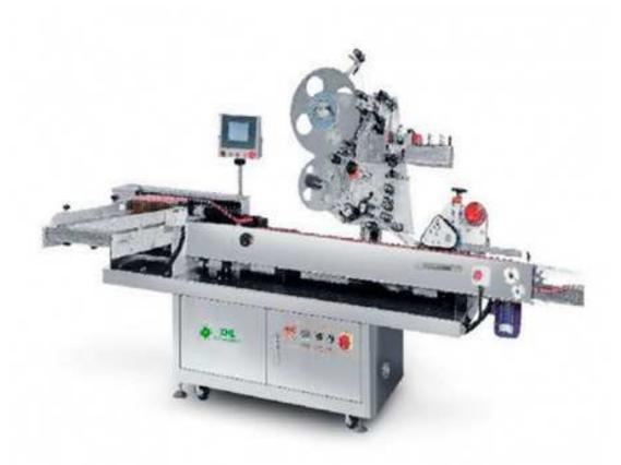
This series machine is applying to glass & plastic bottle. In the field of pharmaceutical, pesticide, chemical, foodstuff etc. It is able to auto separating bottle, feeding label stripe, separating label, sticking and auto printing codes. It is equipped with large torque step motor or servo motor and imported photoelectric controlled PLC to ensure the accuracy, stability, reliability and high efficiency.
