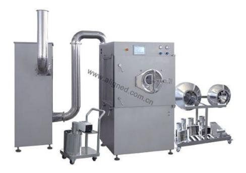
Integral High Efficiency Coating Machine (BG-20H) combines the main machine with the hot air cabinet, air exhaust cabinet, peristaltic pump, printer and control system. It can be widely used for coating various tablets, pills and sweets with organic film, water-soluble film and sugar film etc. In such fields as of pharmaceutical, food and biological products etc. And it has such characteristics as good appearance in design, high efficiency, low energy consumption and small floor area, etc.
