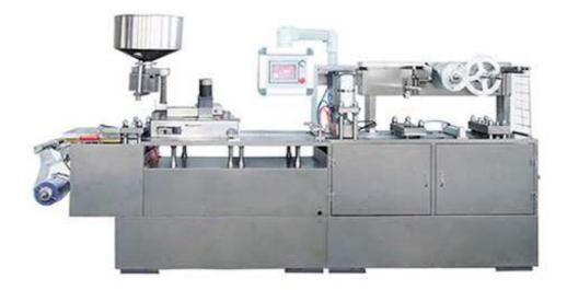
This machine adopts PLC control, man-machine interface operation, frequency conversion speed regulation, high degree of automation and easy operation.
