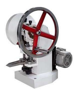
Pill Tablet Press Machine is used for pressing different kinds of granular raw materials into round tablets. Pill Tablet Press Machine is applicable to trial manufacturing in lab or batch production in small amount different kinds of tablets, sugar pieces, calcium tablets and tablets of abnormal shape.
