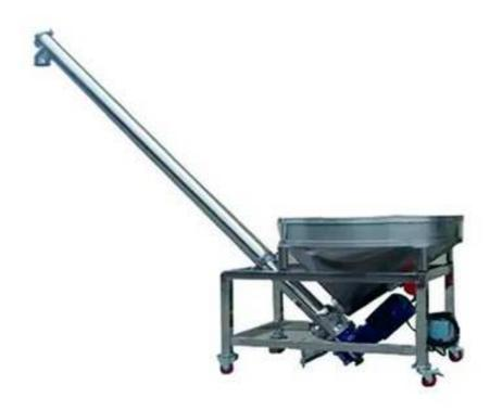
This conveyor is suitable for multiple powder. Working together with packaging machine, the conveyor of the product feeding is controlled to retain the product level in the product cabinet of packaging machine. And the machine can be used independently. All parts are made of stainless steel except the motor, bearing and support frame.
