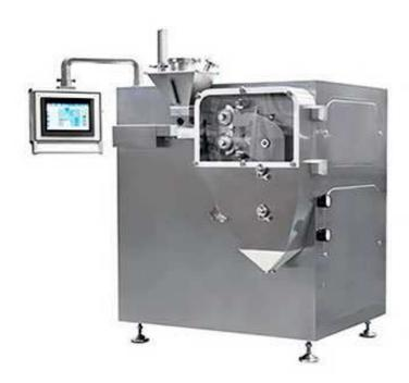
Pharmaceutical dry granulator machine is a kind of environmental protection equipment with low investment, high efficiency, energy saving and no pollution. The process of compacting, forming, crushing and granulator of dry particles by mechanical extrusion is carried out by using the crystalline water of the material itself.
