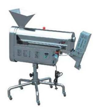
JFP series capsule polisher is a kind of capsule polisher with function of sorter. It plays the function of not only the polishing for capsule and tablet but eliminating static electricity. It can also automatically reject low weight capsule; loose piece and fragments of capsules. It is suitable for all sizes of capsules without the need to change parts.
