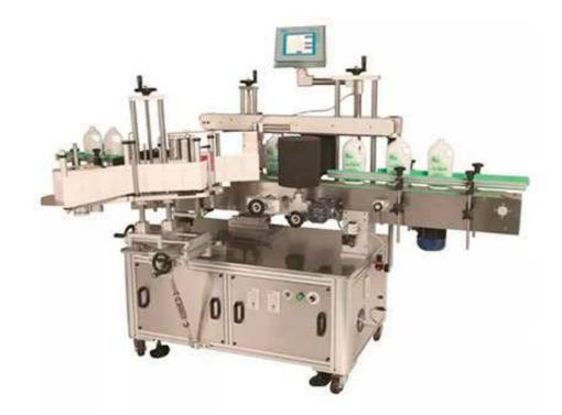
With A Speed Of 6000bph And Various Label Sticking Types (1, 2, 3 Labels), The Linear Type Self-Adhesive Label Sticking Machine Is A Good Choice For The Beverage Filling Production Lines.
