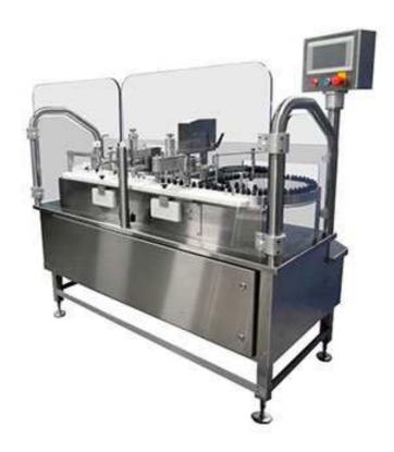
The PallayPack Model AbleBlock is a compact, versatile and full-featured, servo-equipped monoblock for the automatic filling, plugging\*, capping\* and labelling\* of your products (\*when equipped with the required options).
