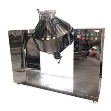
This Mixing Machine is suitable for mixing powder and granular materials in pharmaceutical, chemical, food, building materials and other industries.
