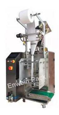
It is suitable for automatic packaging of loose, non-viscous, fine granular and powder material in pharmaceutical and chemical products. Such as activated carbon, charcoal, moxa powder, powder heating packs, herbal medicine powder, aromatherapy, spices, foot powder, Halogen package products, etc.
