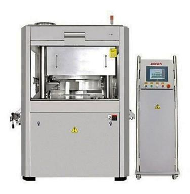
This series of Tablet Press Machines can automatically check, analyze and adjust the pressure to control powder filling depth during tablet production (achieve tablet weight difference between ±2%). It can monitor the progress of punch and die and powder supply, which greatly reduce production costs and increase quality. Adopts a non- hand wheel operation system, which provides a straightforward operation.
