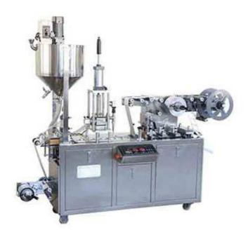
It is suitable for capsule, tablet, big honey pill, candy, liquid, paste, one injector as well as irregular shape AL-PVC, paper-plastic composite and ALU
